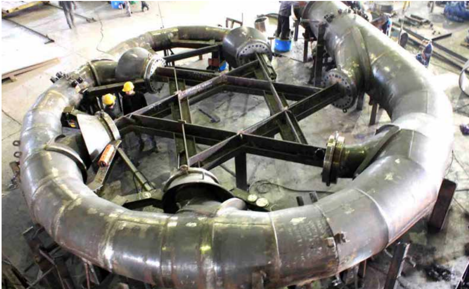
Akköy II Project, Türkiye (2 x 116 MW) Pressure Test 230 Bar / Voith Hydro
